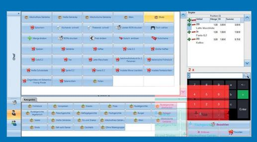
The input screen or keypad of the POS cash register can be freely designed. Here is an example from the gastronomy industry. Depending on industry requirements, functions, products or information fields can be provided in the upper key area.
